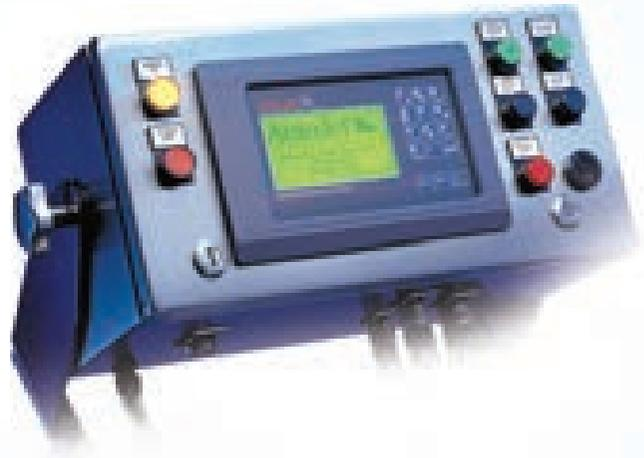
**AutoJet Model 2250 Spray Controller** provides closed-loop control of the liquid pressure and the atomizing air pressure to maintain a consistent application of the release agent. Spray timing is triggered by a proximity sensor which senses the presence of the mold platen.
